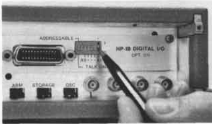
Rear panel switches are set so instrument will either be addressable by controller in a multi-device system, or will simply "talk only" to another device such as a printer or D/A converter.
