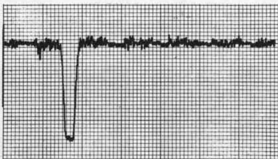
Figure 5b. The difference between a normal system and one that has problems is immediately apparent. One of the channels has dropped out.
