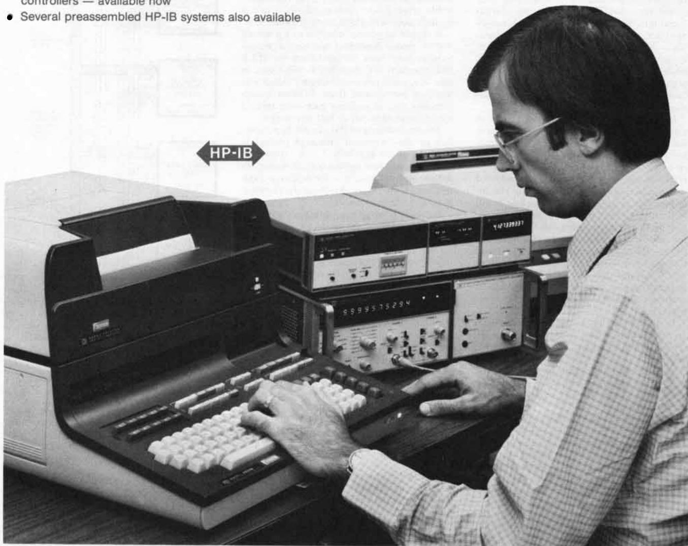
A typical multi-device bench instrument system interconnected via HP-IB, and operating under calculator program control.
